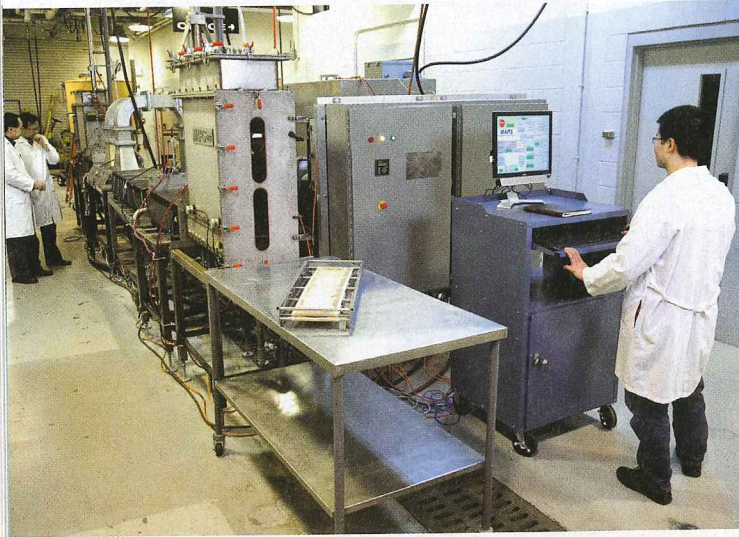
Washington State researchers are adapting a microwave sterilization unit for use in pasteurization under the name MAPS, an acronym for microwave assisted pasteurization system. Photo: Washington State University
